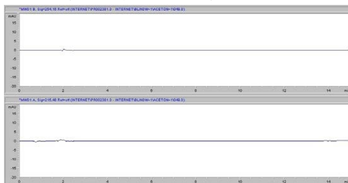
Fig 3. Representative chromatograms of solvents filtered through regenerated cellulose membrane syringe filters and subjected to HPLC analysis. Top panel in each set of chromatograms shows results at 254 nm; bottom panel shows results at 215 nm.
